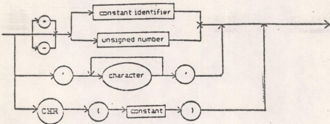
The non-standard CHR construct is provided here so that constants may be used for control characters. In this case the constant in parentheses must be of type integer.
